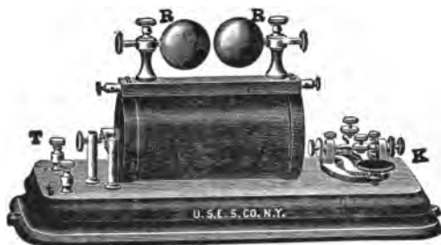
FIG. 58.—Simple Form of Wireless Sending Apparatus for Transmitting to a Distance of a Few Metres.
